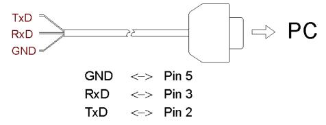
Figure 8: Wiring example for connecting the RS232 interface to a 9 pin D-SUB plug
