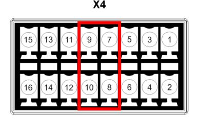
Figure 14: Digital outputs OUT1 / OUT2
