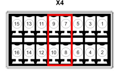
Figure 9: Data-Clock Interface on connector X4
