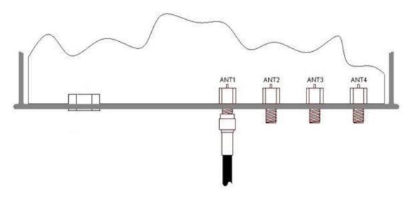
Figure 3: External antenna connection ANT1-4
