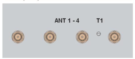
Figure 18: Position of the reset button T1
