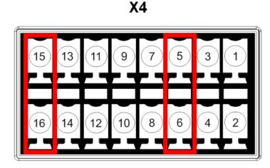
Figure 16: Relay outputs REL1 / REL2
