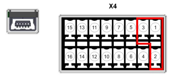
Figure 7: RS232 interface pin-outs on X4
