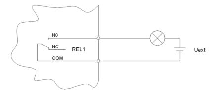
Figure 17: External wiring of the relay outputs
